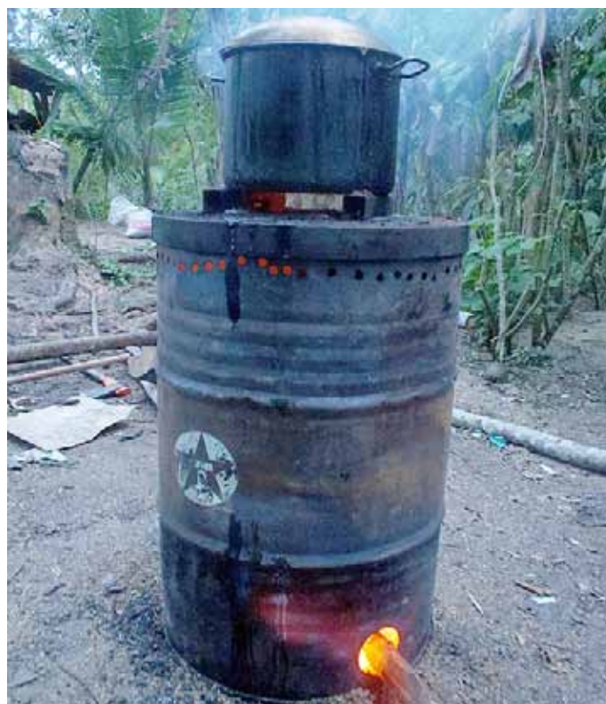
Figure 3. Biochar cook stove constructed by the Maya Mountain Research Farm in Belize
